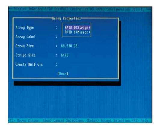
4. The item **"Create RAID via"** allows you to select between the different methods of creating RAID 0 and RAID 1.
